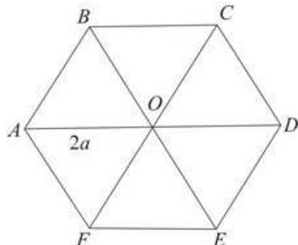
You consider the hexagon to be made up of 6 triangles. Each of the six triangles has the moment of inertia found in part a about the centre of the hexagon  $O$ .
