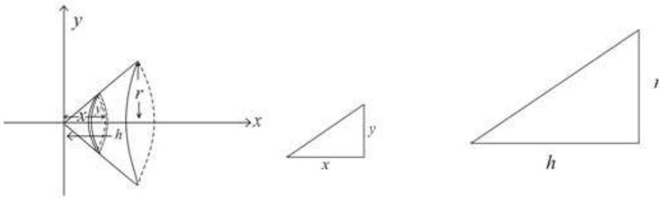
Divide the cone into thin discs – one of which is shown.
