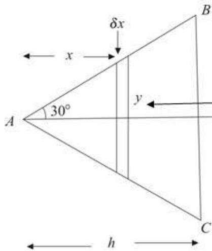
You consider the triangle as made up of thin rods of length  $2y$ , thickness  $\delta x$  and mass  $\delta m$ . A rod is a distance  $x$  from  $A$ .
