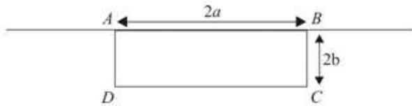
The diagram shows a sign which hangs outside a shop. The sign is a thin rectangular metal plate which is free to rotate about a fixed smooth horizontal axis which lies along the side  $AB$ . The lengths of  $AB$  and  $BC$  are  $2a$  and  $2b$  respectively. The sign can be modelled as a uniform rectangular lamina. The sign is hanging freely below the
