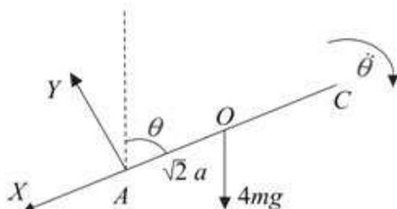
$$\begin{aligned} AO^2 + BO^2 &= AB^2 = (2a)^2 = 4a^2 \\ 2AO^2 &= 4a^2 \Rightarrow AO^2 = 2a^2 \Rightarrow AO = \sqrt{2}a \end{aligned}$$
