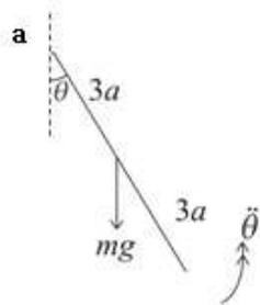
$$\text{M.I. of rod about axis through one end} = \frac{4}{3}m(3a)^2 = 12ma^2$$
