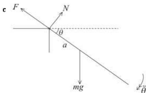
Consider the motion of a particle of mass  $m$  at the mid-point of the rod.
