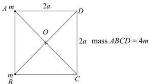
M.I. of lamina and particle about perpendicular axis through O
