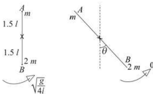
M.I. of loaded rod about given axis
