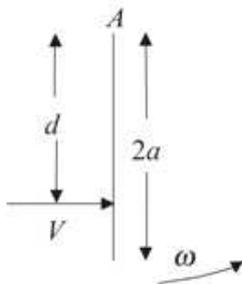
Let the angular speed of the rod and body about  $A$  immediately after the impact be  $\omega$ . Conservation of angular momentum about  $A$
