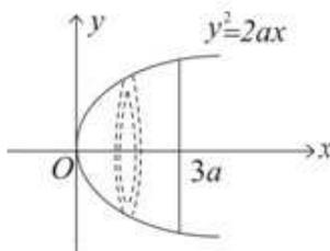
Let the mass per unit volume be  $\rho$ . Divide the solid  $S$  into a large number of thin discs, perpendicular to the  $x$ -axis. A typical disc is shown. This has mass  $\rho\pi y^2 \delta x$  and
