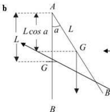
In this diagram, G is the centre of mass of the rod and  $\alpha = \arccos\left(\frac{1}{3}\right)$ .
