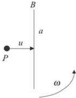
This diagram is drawn looking at the disc edge on.  $\omega$  is the angular speed of the disc and particle immediately after impact.
