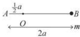
$$\text{Moment of inertia of rod about mid-point} = \frac{1}{3}ma^2$$
