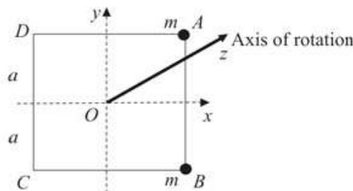
The moment of inertia of the lamina alone about the axis of rotation is given, using the perpendicular axes theorem, by
