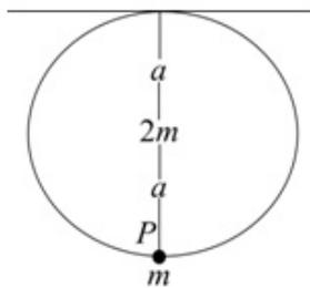
$$\text{Moment of inertia of sphere about diameter} = \frac{2}{5}(2m)a^2$$
