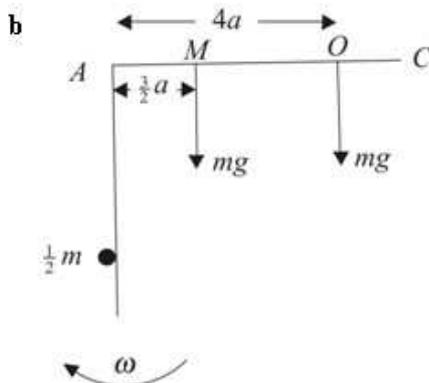
If  $M$  is the centre of mass of the rod and  $O$  is the centre of the mass of the disc, then  $AM = \frac{3}{2} a$  and  $AO = 4a$ .
