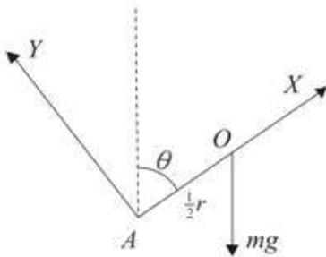
When  $AO$  has rotated through an angle  $\theta$ , let the components of the force parallel and perpendicular to  $AO$  be  $X$  and  $Y$  respectively. Conservation of energy
