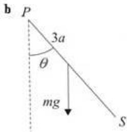
This diagram is drawn viewing the flap from the side. The weight acts at the centre of mass of the lamina.
