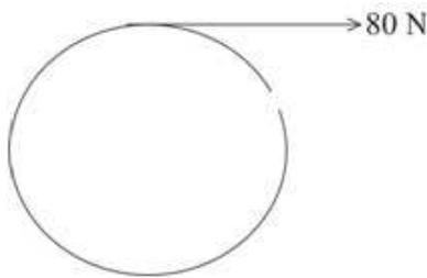
$$\begin{aligned}\text{Work done by the force} &= 80 \times 6 \\ &= 480 \text{ J}\end{aligned}$$
