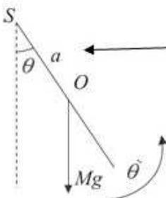
In this diagram, the smooth pivot is  $S$  and the angle  $SO$  makes with the downward vertical is  $\theta$ .
