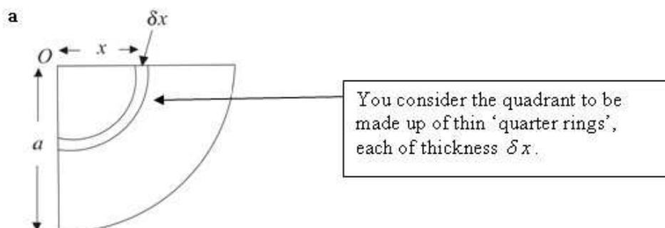
The mass per unit area of the quadrant is  $\frac{m}{\frac{1}{4}\pi a^2} = \frac{4m}{\pi a^2}$
