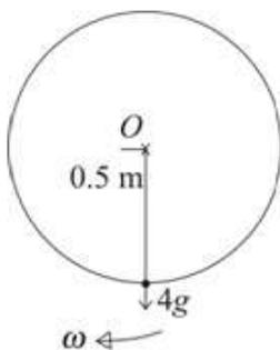
$$\begin{aligned} \text{M.I. of disc + particle about axis through } O &= \frac{1}{2} \times 20 \times (0.5)^2 + 4 \times (0.5)^2 \\ &= 3.5 \text{ kg m}^2 \end{aligned}$$
