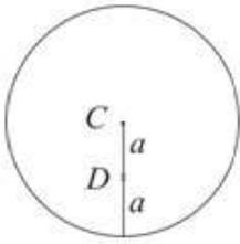
M.I. of disc about axis through  $C = \frac{1}{2}m(2a)^2 = 2ma^2$
