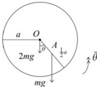
$$\begin{aligned} \text{M.I. of disc and particle about axis at } O &= \frac{1}{2} \times 2ma^2 + m \times \left(\frac{1}{2}a\right)^2 \\ &= \frac{5}{4}ma^2 \end{aligned}$$
