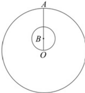
A uniform disc of mass  $3m$  has centre  $O$  and radius  $3a$ . A disc with centre  $B$  and radius  $a$  is removed. The line  $OB = a$  and, when produced, meets the circumference of the larger disc at  $A$  as shown in the diagram. The remaining lamina is free to rotate about a fixed smooth horizontal axis which coincides with the tangent to the disc at  $A$ .
