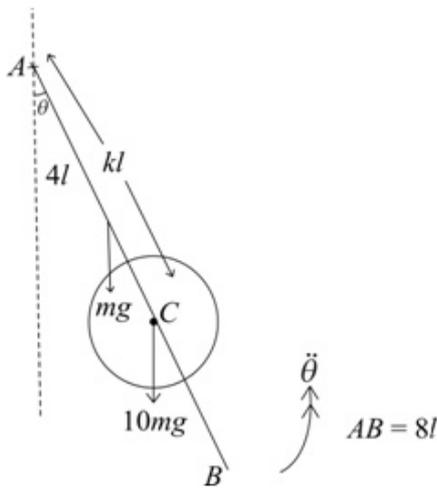
M.I. of rod and disc about axis at A
