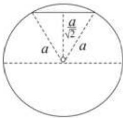
The moment of inertia of the sphere about a diameter  $= \frac{2}{5} ma^2$
