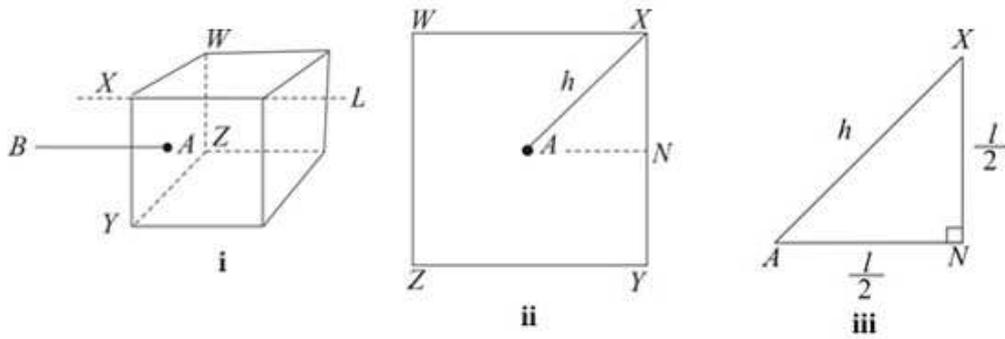
Diagram **i** shows the rod  $AB$  attached at  $A$ , the centre of the face  $WXYZ$ . It also shows the axis  $L$  through point  $X$  perpendicular to face  $WXYZ$ .
