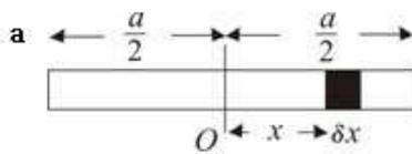
You consider the rod to be made up of a series of small pieces, or elements, each of length  $\delta x$ .
