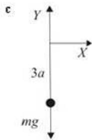
When writing down an equation of motion, you consider the whole mass of the lamina to be at the centre of mass of the lamina, which is  $3a$  from the axis of rotation.
