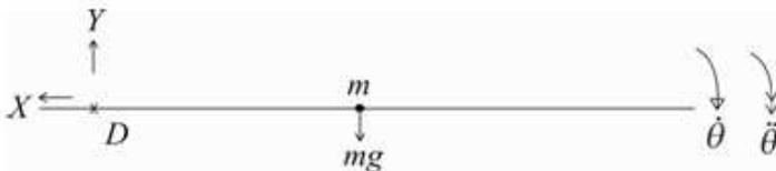
Consider the motion of a particle of mass  $m$  at the centre of mass of the disc:
