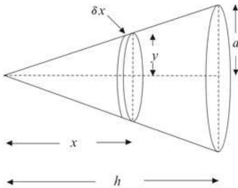
You consider the cone to be made up of thin discs, each of thickness  $\delta x$  with the centre of the disc at a distance  $x$  from the vertex of the cone. If the radius of the disc is  $y$ , then, using the formula,  $V = \pi r^2 h$ , for the volume of a cylinder, the volume of a thin disc is  $\pi y^2 \delta x$ .
