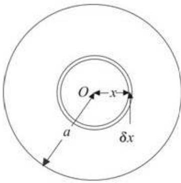
You consider the disc as made up a series of concentric rings of thickness  $\delta x$ . The area of each ring is  $2\pi x\delta x$ .
