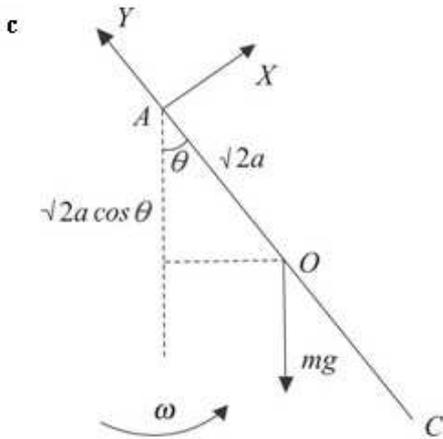
Let  $X$  and  $Y$  be the components, perpendicular to and along  $AC$ , of the reaction of the lamina on the axis.
