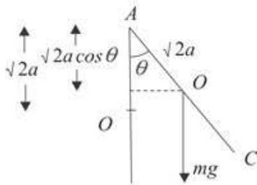
As the lamina swings through an angle  $\theta$  with the vertical, the centre of mass falls a distance of  $\sqrt{2}a - \sqrt{2}a \cos \theta$ .
