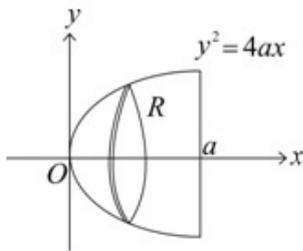
Divide  $S$  into discs parallel to the circular base of the solid let the mass per unit volume be  $\rho$ .
