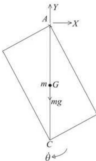
Consider the motion of a particle of mass  $m$  placed at the centre of mass of the framework.
