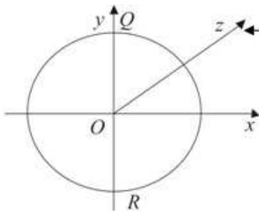
The standard result for the moment of inertia of a disc  $\left( I = \frac{1}{2}ma^2 \right)$  is for an axis through its centre perpendicular to the plane of the disc. From this you need to find the moment of inertia about a diameter. You then use the moment of inertia about a diameter to find the moment of inertia of the disc about  $L$ .
