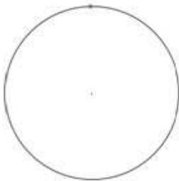
$$\begin{aligned} \text{M.I. of hoop about perpendicular axis through its centre} &= mr^2 \quad \leftarrow \text{From the formula book.} \\ &= 1.2 \times 1.5^2 \text{ kg m}^2 \end{aligned}$$
