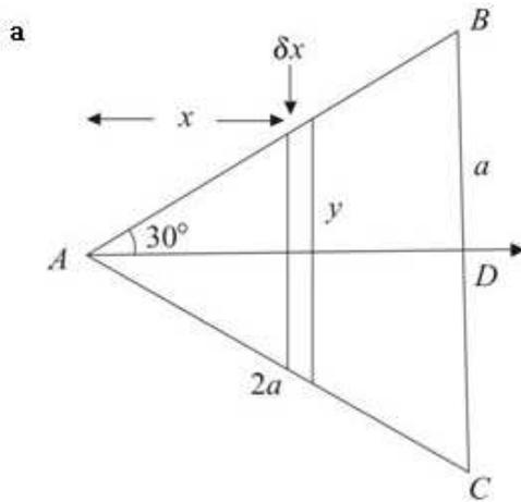
You consider the triangle as made up of thin rods of length  $2y$ , thickness  $\delta x$  and mass  $\delta m$ . The rod is a distance  $x$  from  $A$ .
