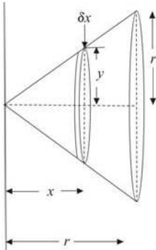
You consider the cone to be made up of thin discs, each of thickness  $\delta x$  with the centre of the disc at a distance  $x$  from the vertex of the cone. If the radius of the disc is  $y$ , then, using the formula,  $V = \pi r^2 h$ , for the volume of a cylinder, the volume of a thin disc is  $\pi y^2 \delta x$ .
