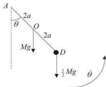
The moment of inertia of the compound pendulum,  $I$ , about the axis through  $A$  is given by
