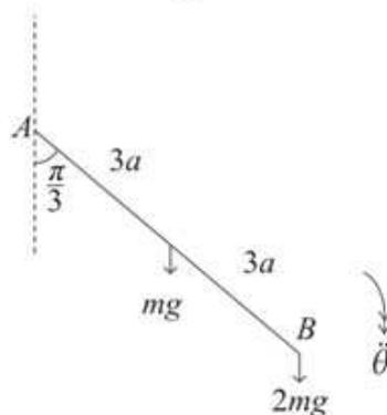
$$mg \times 3a \sin \frac{\pi}{3} + 2mg \times 6a \sin \frac{\pi}{3} = 84ma^2 \ddot{\theta}$$
