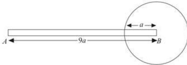
A pendulum  $P$  is modelled as a uniform rod  $AB$ , of length  $9a$  and mass  $M$ , rigidly fixed to a uniform circular disc of radius  $a$  and mass  $2M$ . The end  $B$  of the rod is attached to the centre of the disc and the rod lies in the plane of the disc as shown in the figure. The pendulum is free to rotate in a vertical plane about a fixed smooth horizontal axis  $L$  which passes through end  $A$  and is perpendicular to the plane of the disc.
