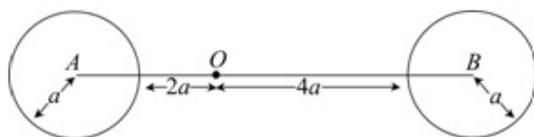
A body consists of two uniform circular discs, each of mass  $m$  and radius  $a$ , with a uniform rod. The centres of the discs are fixed to the ends  $A$  and  $B$  of the rod, which has mass  $3m$  and length  $8a$ . The discs and the rod are coplanar, as shown in the figure. The body is free to rotate in a vertical plane about a smooth fixed horizontal axis. The axis is perpendicular to the plane of the discs and passes through the point  $O$  of the rod, where  $AO = 3a$ .
