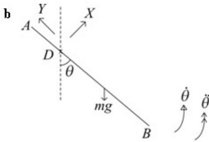
$\dot{\theta}$  and  $\ddot{\theta}$  are in the direction of increasing  $\theta$ .
