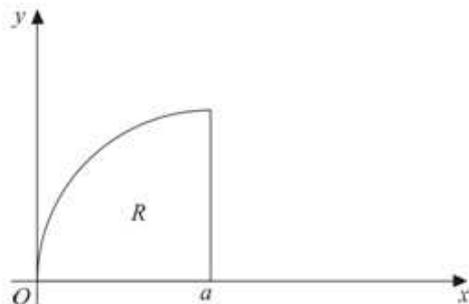
A region  $R$  is bounded by the curve  $y^2 = 4ax$  ( $y > 0$ ), the  $x$ -axis and the line  $x = a$  ( $a > 0$ ), as shown. A uniform solid  $S$  of mass  $M$  is formed by rotating  $R$  about the  $x$ -axis through  $360^\circ$ . Using integration, prove that the moment of inertia of  $S$  about the  $x$ -axis is  $\frac{4}{3}Ma^2$ . ***E***
