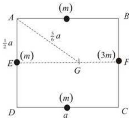
If  $E$  is the mid-point of  $AD$  and  $F$  is the mid-point of  $BC$ , then, by symmetry, the centre of mass of the framework  $G$  lies on  $EF$ . The location of  $G$  is found by taking moments about  $E$ .
