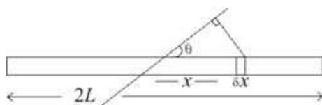
Divide the rod into small pieces of length  $\delta x$  at a distance  $x$  along the rod from the middle. The perpendicular distance from the small piece shown to the axis is  $x \sin \theta$ , where  $\theta$  is the constant given angle.
