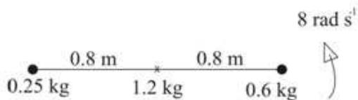
M.I. of rod and particles about the given axis through the mid-point
