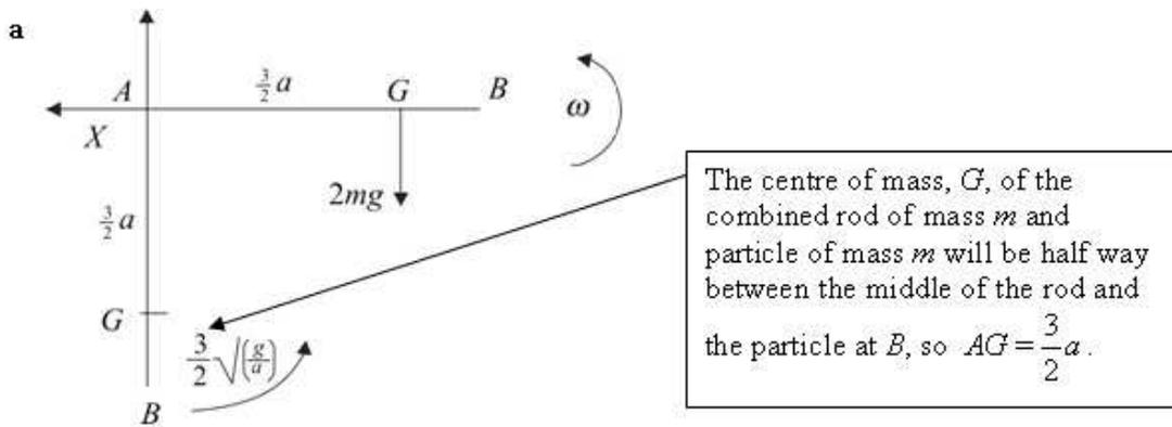
The moment of inertia of the combined rod and particle about  $A$  is given by
