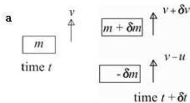
$$(m + \delta m)(v + \delta v) + (-\delta m)(v - u) - mv = -mg \delta t$$
