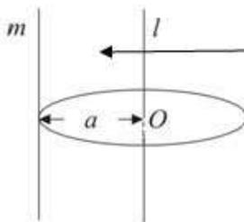
In part a, you have shown that the moment of inertia about the axis  $l$ , an axis through the centre perpendicular to the plane of the disc, is  $\frac{1}{2}Ma^2$ . You find the moment of inertia about the axis  $m$ , an axis parallel to  $l$ , through a point on the circumference of the disc, using the result of part a and the parallel axes theorem.
