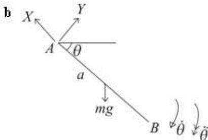
Consider the motion of a particle of mass  $m$  at the centre of mass of the rod.
