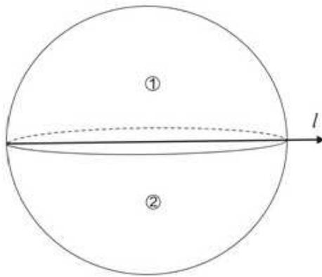
If you consider a complete sphere as being made up to two hemispheres, then, by the addition rule, the sum of the moments of inertia of the two hemispheres about the axis  $l$ , in this diagram, must equal the moment of inertia of the whole sphere about  $l$ . So a hemisphere has half the moment of inertia of the whole sphere. However, the mass  $m$  is not now the mass of the whole sphere and you must be careful to avoid the incorrect answer  $\frac{1}{5}mr^2$ .
