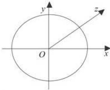
By the perpendicular axes theorem, the moment of inertia,  $I_{Ox}$ , about a diameter  $Ox$  through  $O$  is given by
