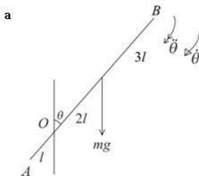
$$\begin{aligned} \text{M.I. of rod about axis through } O &= \frac{1}{3}m(3l)^2 + m(2l)^2 \\ &= 7ml^2 \end{aligned}$$
