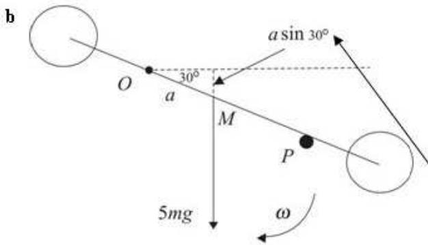
As the body rotates through  $30^\circ$ , the centre of mass of the body,  $M$ , falls vertically a distance  $a \sin 30^\circ = \frac{1}{2}a$ .
