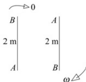
$$\begin{aligned} \text{a P.E. lost} &= mgh = 2.5 \times 9.8 \times 1 \\ &= 24.5 \end{aligned}$$
