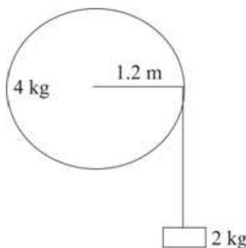
$$\begin{aligned} \text{P.E. lost by block} &= 2g \times 5 \\ &= 98 \text{ J} \end{aligned}$$
