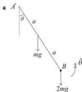
$$\text{M.I. of rod and particle about axis at } A = \frac{4}{3}ma^2 + 2m(2a)^2$$
