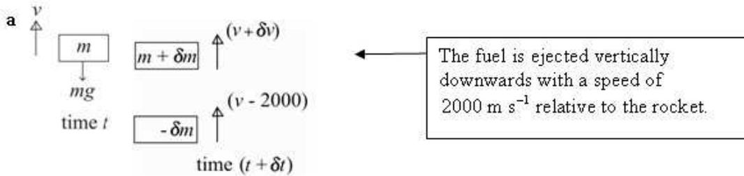
The fuel is ejected vertically downwards with a speed of  $2000 \text{ m s}^{-1}$  relative to the rocket.
