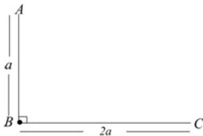
As the wire is uniform, mass of  $AB$  is  $\frac{m}{3}$  and mass of  $BC$  is  $\frac{2m}{3}$ .
