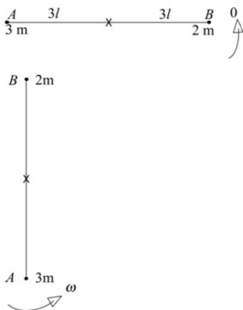
M.I. of rod and particles about given axis
