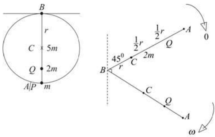
M.I. of disc about perpendicular axis through C
