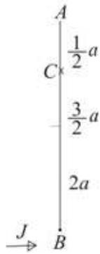
M.I. of rod about axis through  $C = \frac{1}{3}m \times (2a)^2 + m\left(\frac{3}{2}a\right)^2$  ← From the formula book and using the parallel axes theorem.
