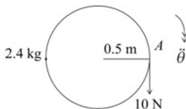
$$\begin{aligned} \text{a M.I. of disc} &= \frac{1}{2} \times 2.4 \times 0.5^2 \\ &= 0.3 \text{ kg m}^2 \\ 10 \times 0.5 &= 0.3 \ddot{\theta} \\ \ddot{\theta} &= \frac{10 \times 0.5}{0.3} = \frac{50}{3} \end{aligned}$$
