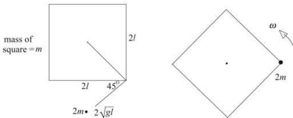
M.I. of square lamina about perpendicular axis through centre
