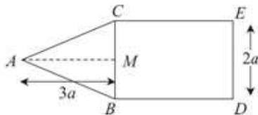
The figure shows a uniform plane lamina of mass  $6m$  formed by joining a triangular lamina  $ABC$  to a rectangular lamina  $BDEC$  along a common line  $BC$ . The sides  $BD$  and  $CE$  are each of length  $3a$ . The side  $DE$  is of length  $2a$ .  $AB = AC$  and  $AM = 3a$ , where  $M$  is the mid-point of  $BC$ . The lamina can rotate about a smooth fixed axis through  $A$ , perpendicular to the plane of the lamina.
