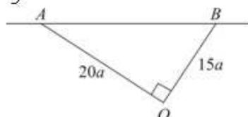
The figure shows a rigid body consisting of two uniform rods. Rod  $AO$  has mass  $m$  and length  $20a$  and the rod  $BO$  has mass  $m$  and length  $15a$ . They are rigidly joined together at  $O$  so that angle  $AOB$  is a right angle. The body is free to rotate about a fixed horizontal axis  $AB$  and hangs in equilibrium with  $O$  below  $AB$ . A particle of mass  $\frac{1}{3}m$  is moving horizontally at right angles to the plane  $OAB$  with speed  $u$ . It
