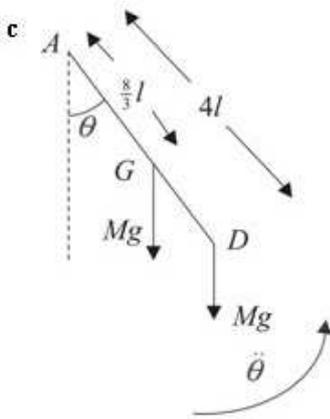
Using the standard result that the centre of mass of a triangle is  $\frac{2}{3}$  along the median from the vertex, if  $G$  is the centre of mass of the triangle then  $AG = \frac{2}{3} \times 4l = \frac{8}{3}l$ .
