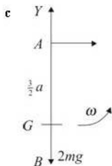
Let the magnitude of the vertical component of the force acting on the rod at  $A$  immediately after the impact be  $Y$ .
